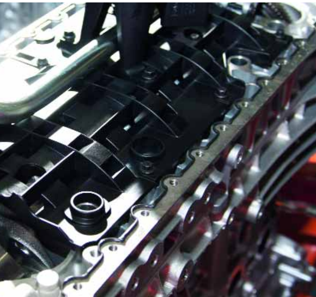
Oil pan joint on a Volvo S16 engine using Loctite 5900 silicone
