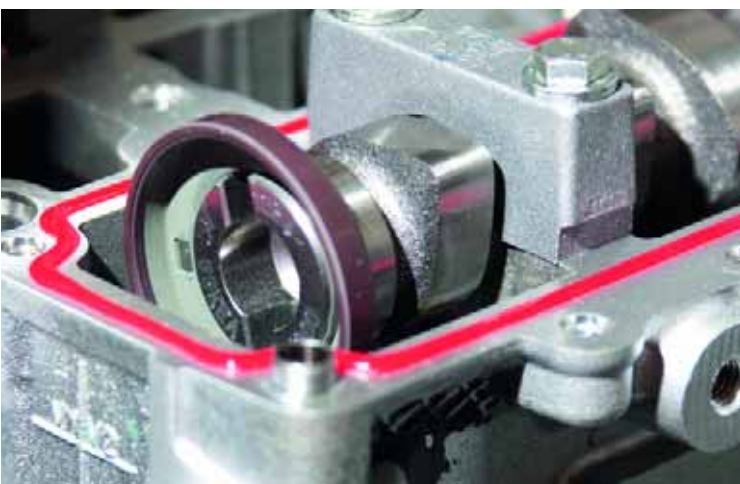
Highly flexible anaerobic Loctite 5188 is used to seal the fuel pump cover on a Sigma engine.
