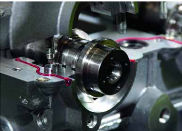
The complex sealing pattern created during cam cap sealing on the Ford Sigma Engine is achieved using 5182 anaerobic sealer applied with a robot.
